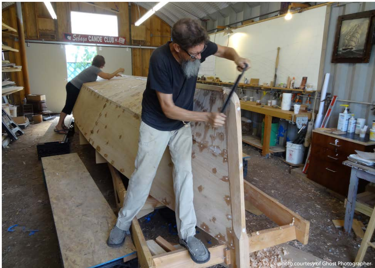
Above: Carving the stem. Below: Running the keel fillet.
