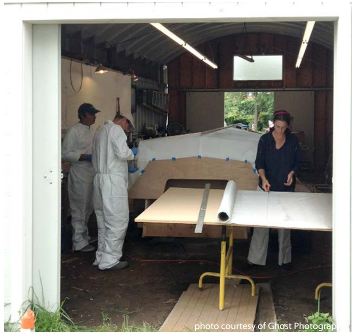
Left: Glassing the hull. Above: Lynn cuts the fiberglass cloth. Below: Wetting out.
