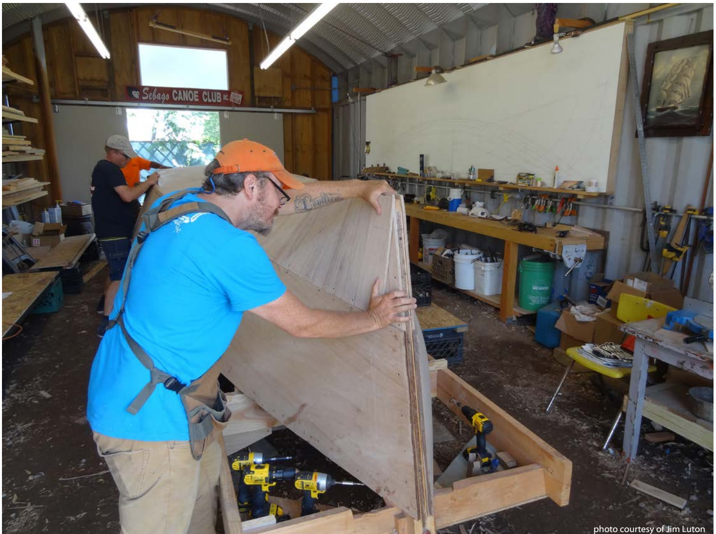
Below: Dry fitting the bow planking.
