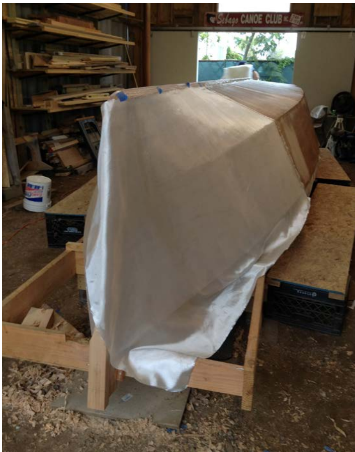
Left: Glassing the hull. Above: Lynn cuts the fiberglass cloth. Below: Wetting out.
