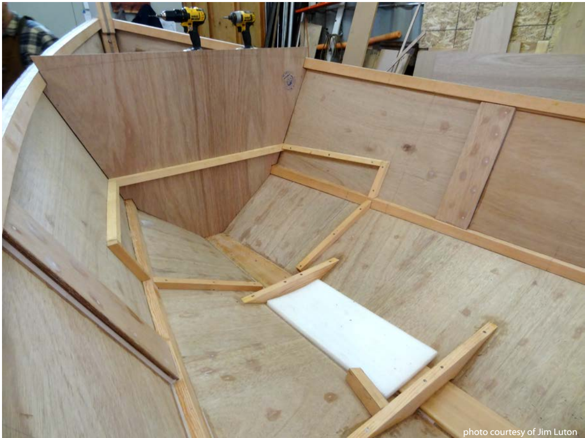
Top: Fitting a locker part. Bottom: Forward bulkhead and anchor locker framing.
