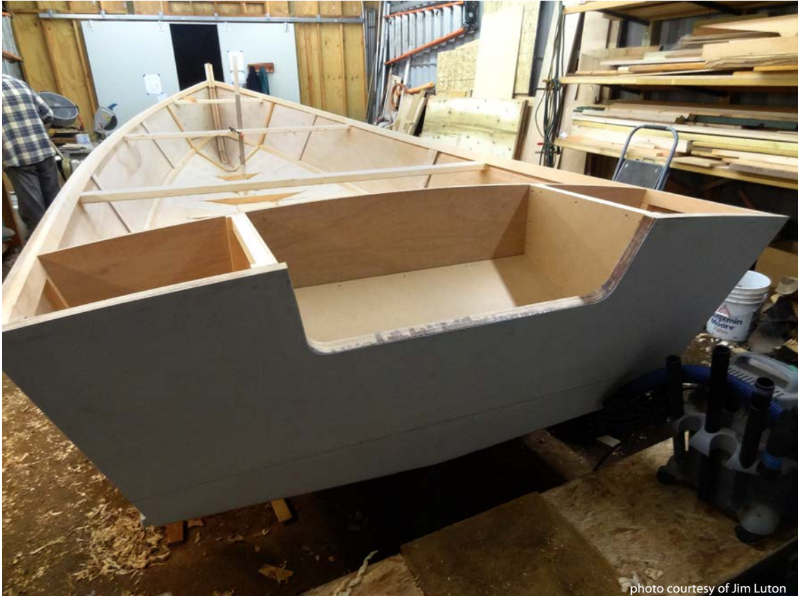
Top: Splash well framing. Bottom: The completed well.
