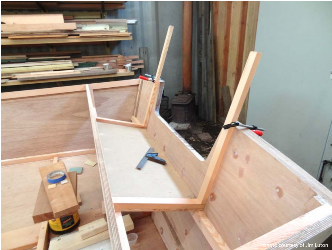
Top: Splash well framing. Bottom: The completed well.
