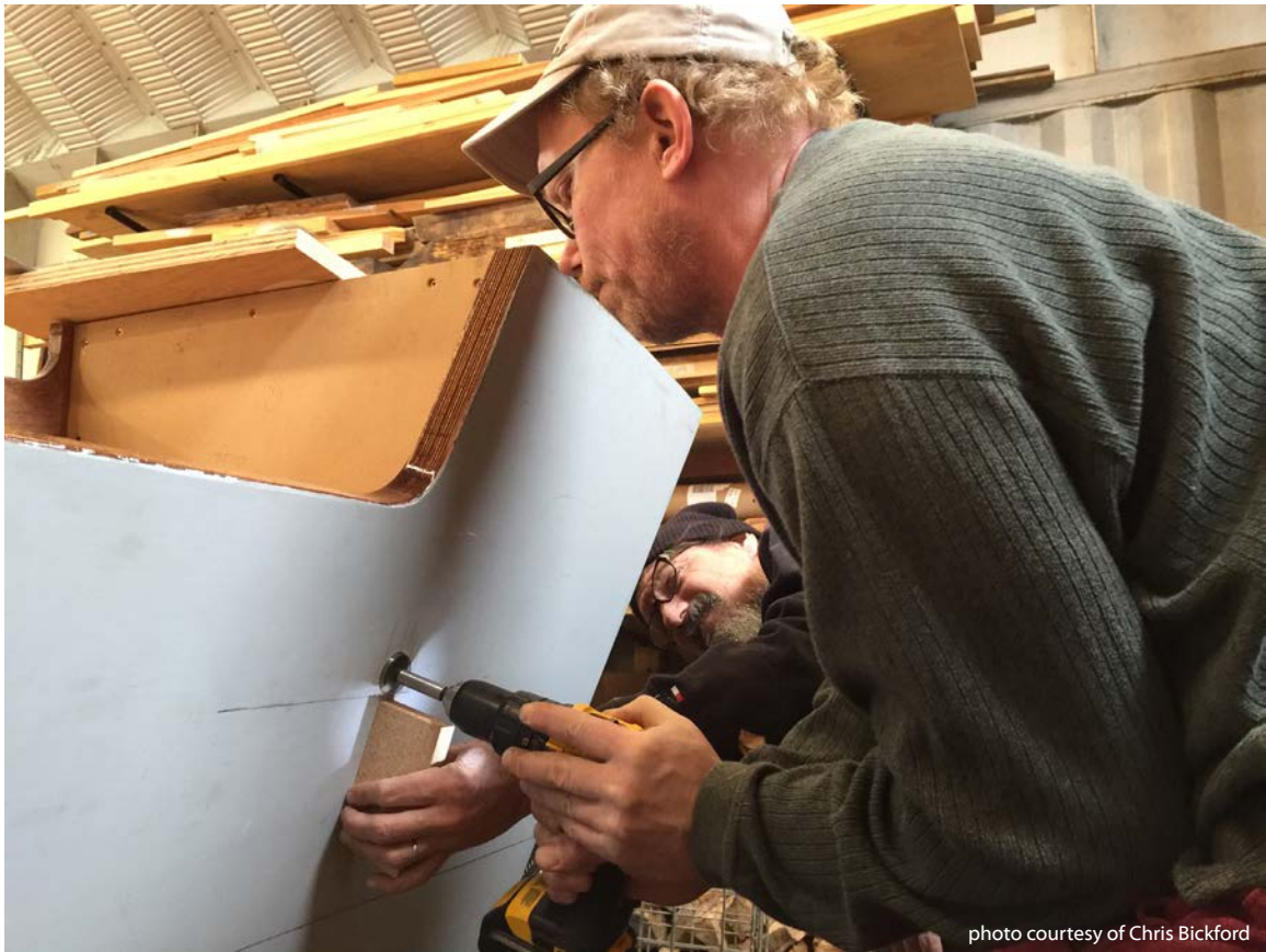
Top: Boring the splash well drains. Bottom: Bulkhead pattern.
